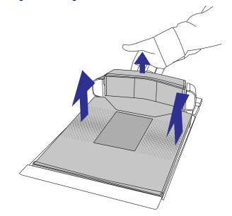
2. The scanner provides lift handles that must be rotated up into position for use as shown in Figure 20. When released, these handles should be allowed to rotate back down into their seated positions in the cavity. Use reasonable care when attempting to lift the unit using any features other than the lift handles.
