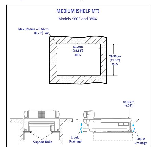
Figure 8. Counter Cutout and Scanner Support Dimensions - Medium
