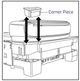
2. For 7" or 12" models, gently slide the Filler Tab from the Corner Piece. This will leave an opening for the neck of the TDR. [For the 9" model, use the new Corner Piece provided.]
