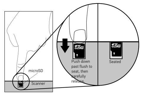
5. If installed properly, you should immediately hear an audible signal upon insertion or removal of a microSD card. Various operations will also be indicated by the scanner's good read LED.
