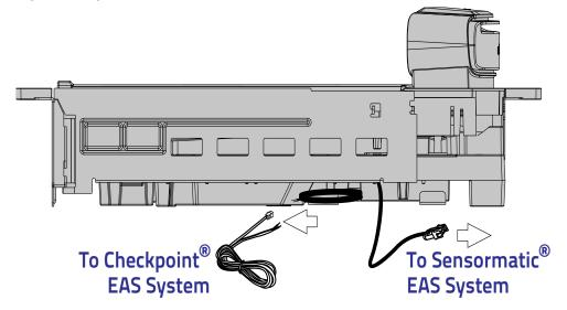
5. Make sure that all cables are firmly attached (except the AC/DC power supply, which should not be connected to the AC outlet yet).
