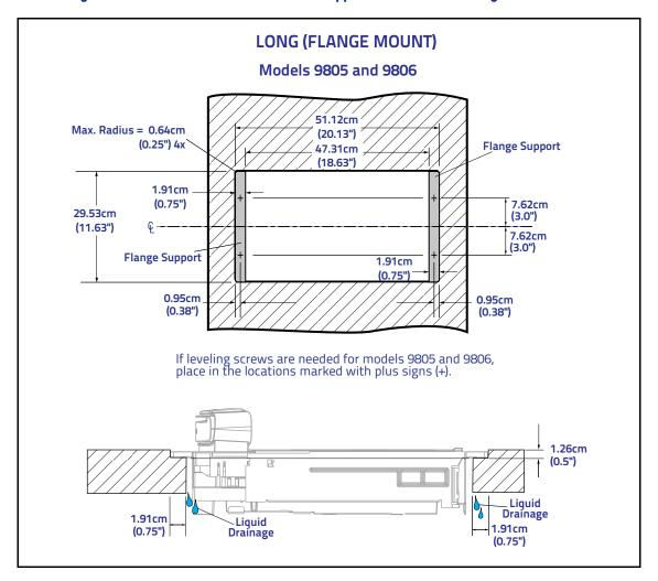
Figure 9. Counter Cutout and Scanner Support Dimensions - Long
