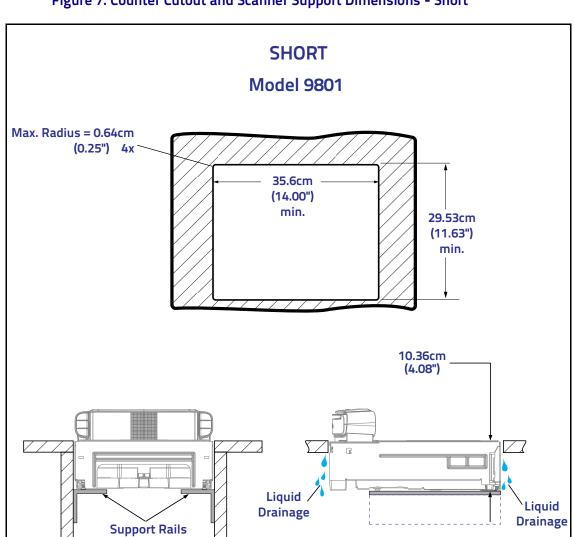
Figure 7. Counter Cutout and Scanner Support Dimensions - Short
