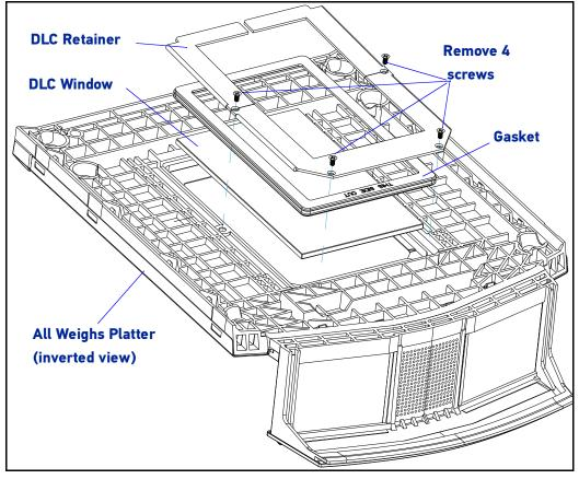
9. Reinstall the platter to complete the process.
