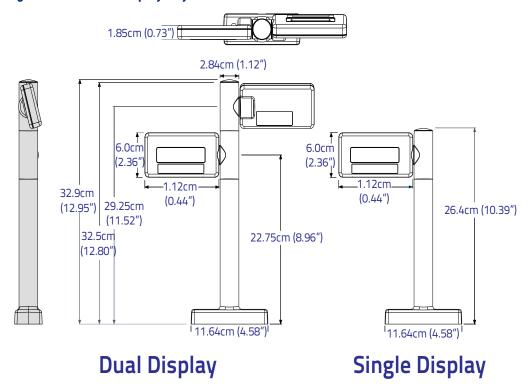
Figure 22. Remote Display Physical Measurements
