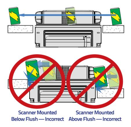
Scanner Mounted Flush — Correct
