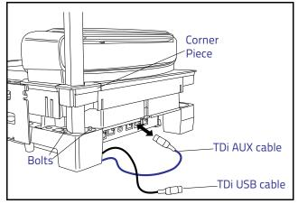
7. Connect the USB cable to the device that will control the TDi. This is typically a PC or POS.
